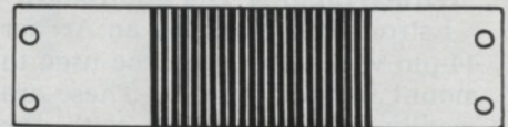
Figure 7. Printed circuit board for buss extension. The use of 1/8 inch adhesive layout tape simplifies the etching process.
